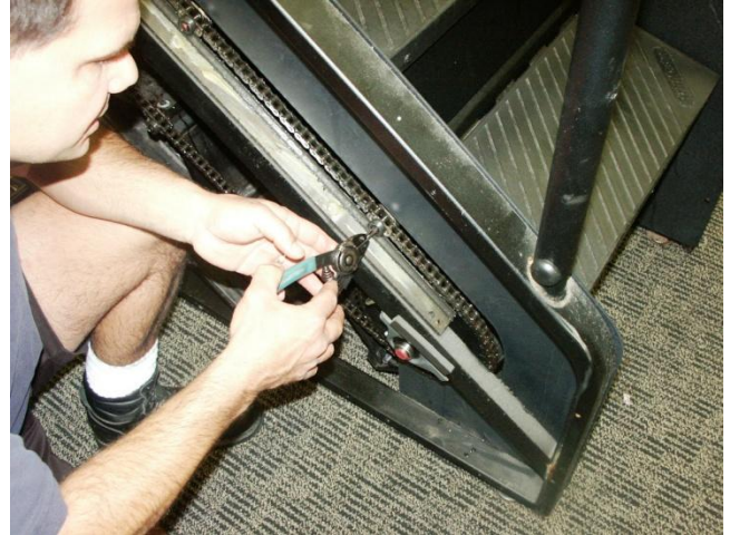
Figure 3. Removing the Snap Ring, Bearing and Flat Washers from the Step Shaft
