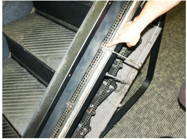
Figure 8. Leaving the Attaching Hardware Intact, Pull the Shaft through from the Right Side
