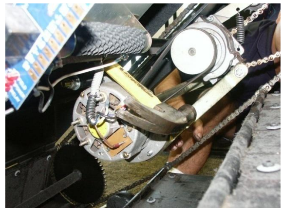
Figure 7. Hammer Providing Belt Tension
