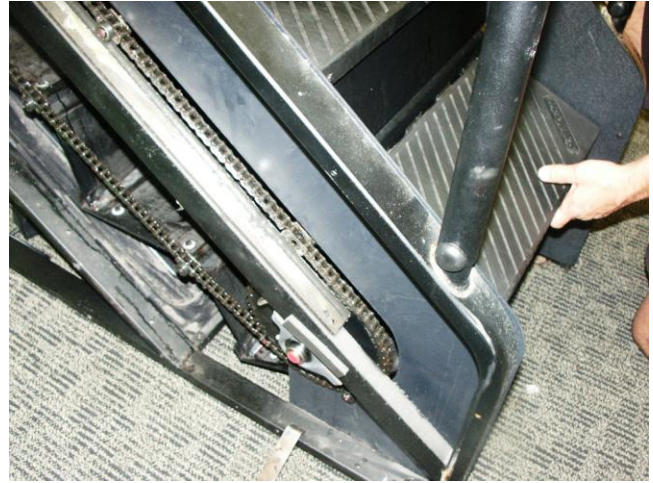
Figure 12. Reinstalling the Step Shaft
