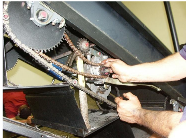
Figure 12. Re-Installing the Back Section of the Master Link
