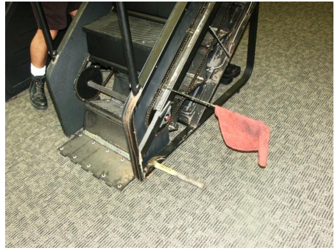
Figure 7. Ready to Replace the Tread Step Cover
