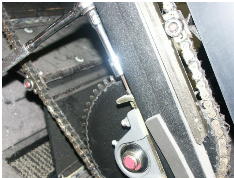
Figure 4. Backing Out the Chain Tensioning Set Screws
