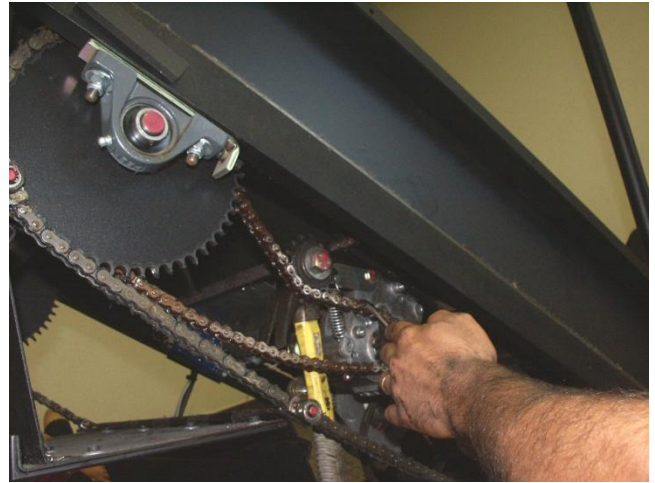
Figure 14. Re-install the Master Link Clip, with the Closed End facing Aft – the Direction of Motion
