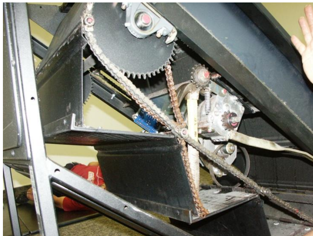
Figure 11. Idler moved to and Held at Max Up Position by Using Your Knee
