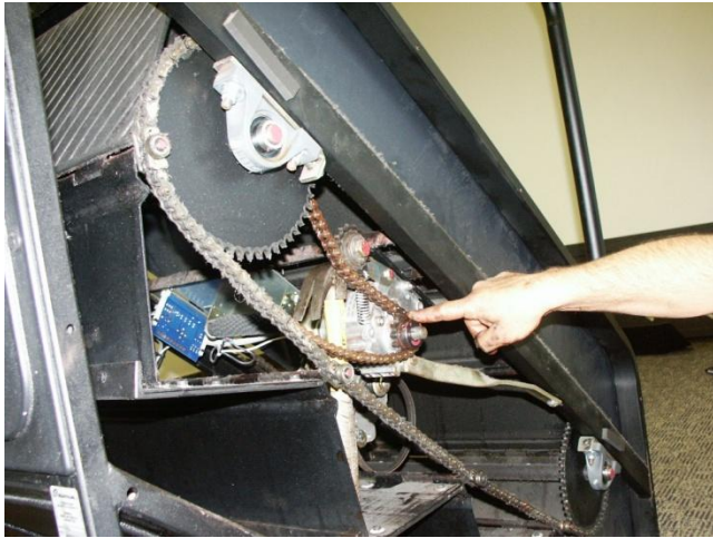
Figure 13. Using Your Knee, Carefully Rotate the Steps Down, Engaging the Idler Sprocket onto the Drive Chain
