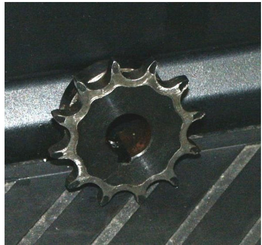
Figure 5A. Sprocket with Excessive Wear - Replace
