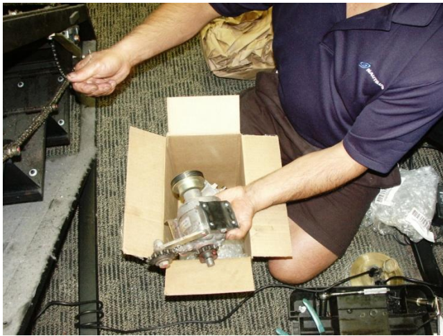
Figure 13. Hardware Installed on New Transmission
