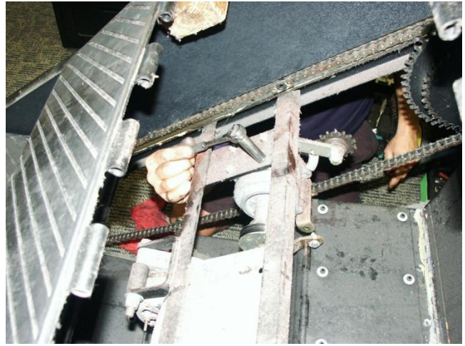
Figure 10. Moving the Steps Aside for Access to the Transmission Mounting Bolts.
