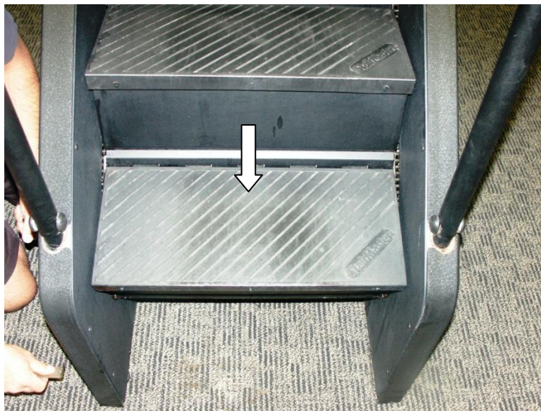
Figure 2. Tread Step Cover to be Replaced
