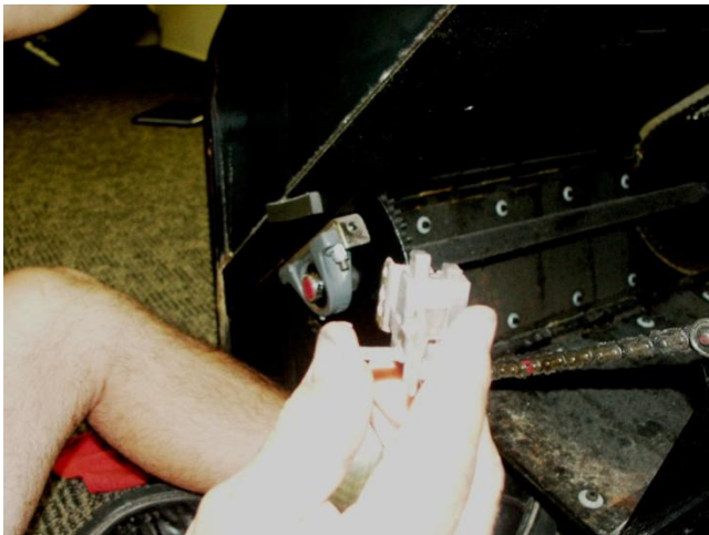
Figure 3. Inspect the Brushes – Note that the Inboard Brush Normally Wears More than the Outboard Brush
