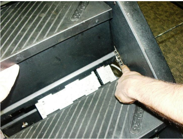
Figure 9. Removing the Shaft and Catching Right Side Inboard Flat Washer
