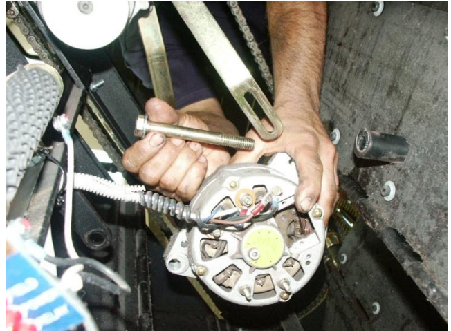
Figure 2. Preparing to Disconnect the Alternator Wires
