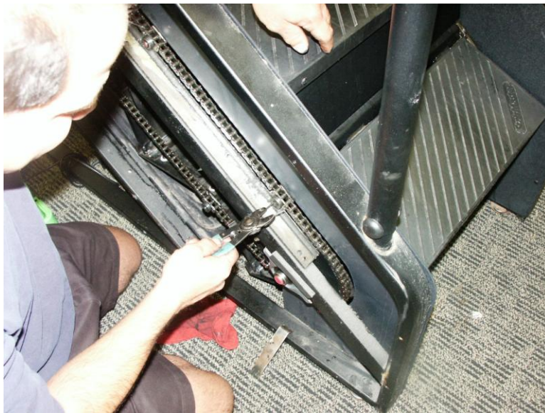
Figure 13. Reinstalling the Bearing and Snap Ring
