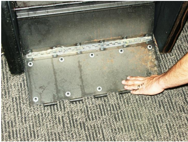
Figure 6. Laying the Step onto the Floor Work Surface
